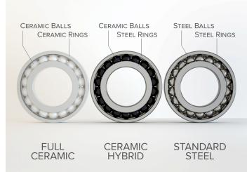
have the longest service life, they also cost up to seven times more than steel bearings. And then there are ceramic hybrid bearings—offering a balance between cost and performance, as they last a minimum of twice as long as full-steel bearings (and often much longer)—at roughly just twice the cost of full-steel bearings they can balance that ratio of performance to cost.
